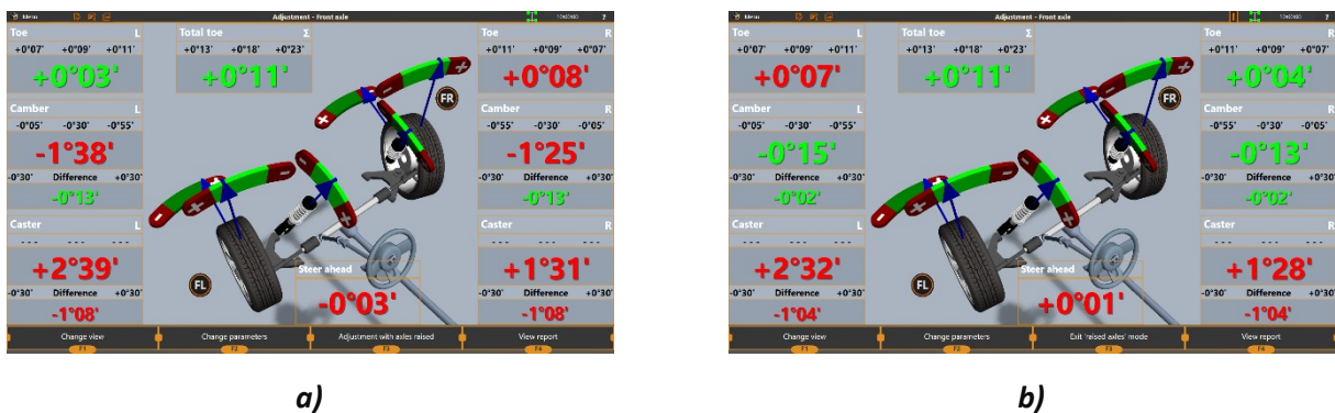
Figure 3.48 – Wheel alignment values for the same wheel position a) in the basic adjustment mode; b) in the suspended wheels mode
