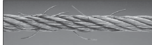
Cable with Broken Wires
